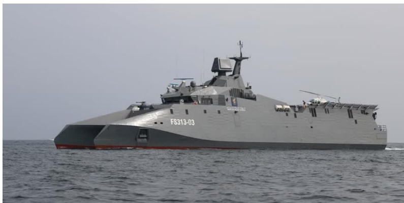
In the picture: “Shahid Shirazi” (FS313-03). A radar array was installed on this ship, apparently in order to improve the ability to create an image of the situation around the ship.
