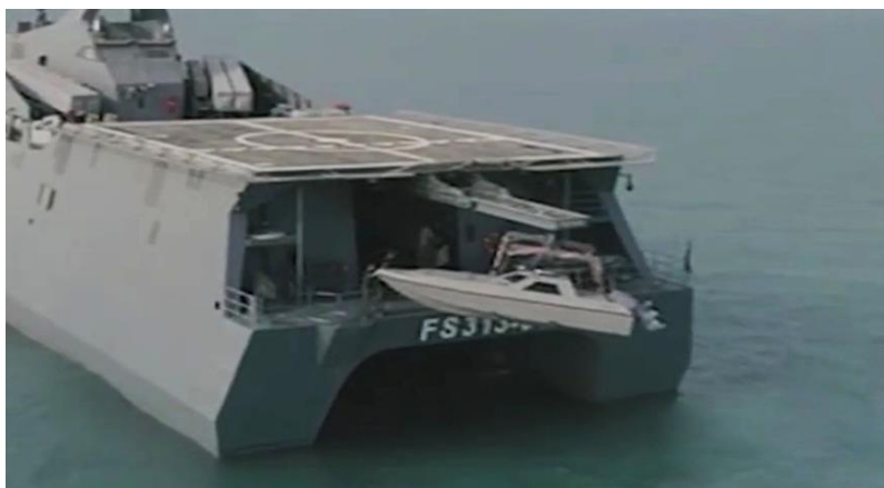
In the picture: Unloading of a speedboat using a crane from a hangar at the stern of the ship
